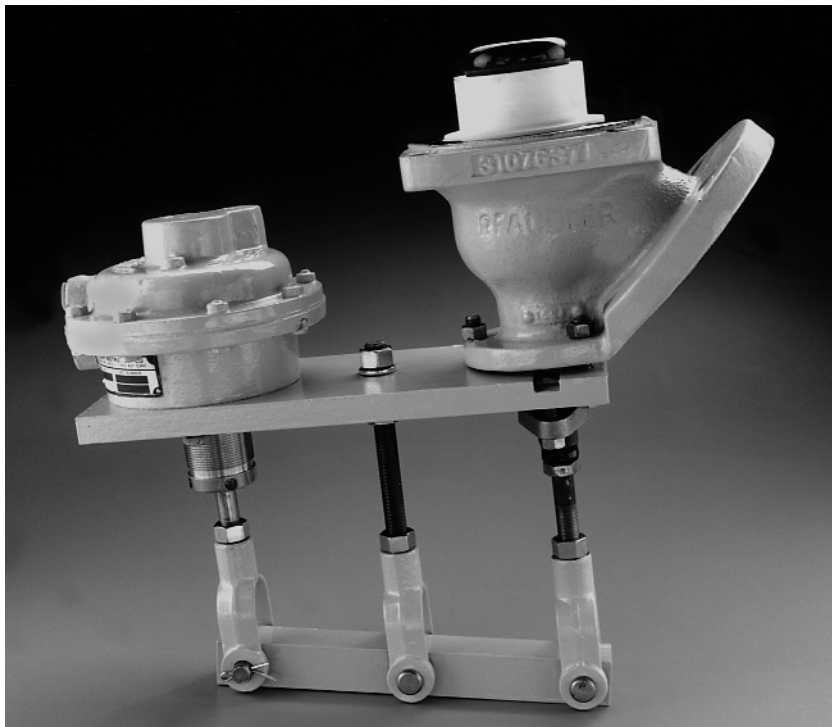
Figure 2: Low-profile, air-actuated flush valve mounts on reactor's bottom outlet nozzle; requires minimal clearance beneath the vessel.
