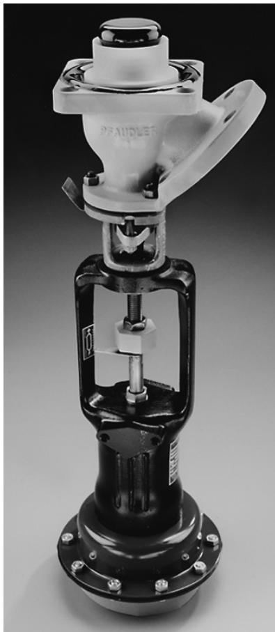
Figure 3: Vertically mounted, air-actuated flush valve with straight-through actuation, suitable for reactors with adequate clearance below the bottom outlet.
