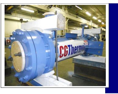
Coupled with our unique "no load" tubesheet the aforementioned properties result in a unit that has exceptional mechanical shock resistance and is 100% immune to thermal shock.
